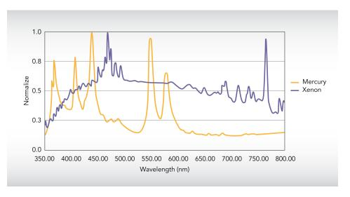
▲ Xenon vs high pressure Mercury lamps
