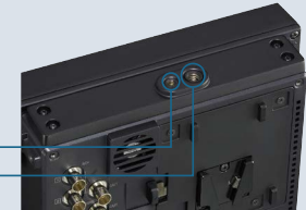
Arm-mount bracket is attached on the top
