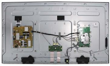
And then remove wifi bracket & speakers with hand and screw driver.
