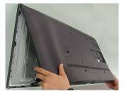
Once removed this will expose the accessible electronic units (PCBs), which can now be easily removed with hand and screw driver.
