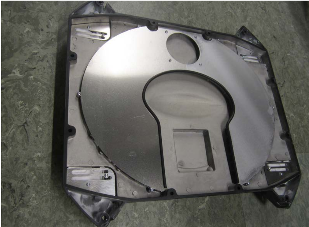
Photo 9. IP6X No dust observed inside the G-Spot Moving Head Profile.
