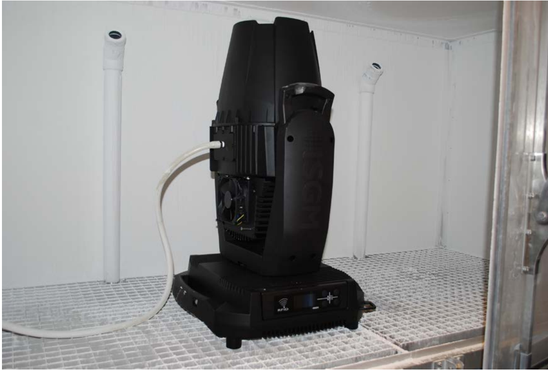
Photo 1. IP6X Test G-Spot Moving Head Profile before exposure.
