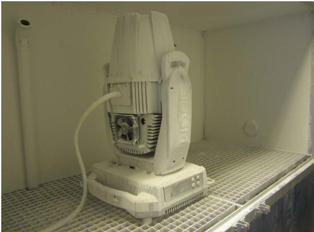
Photo 2. IP6X The G-Spot Moving Head Profile after exposure.
