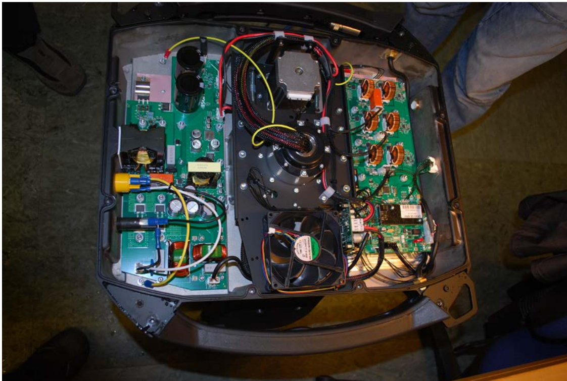
Photo 20. IPX5 No water observed inside the G-Spot Moving Head Profile.
