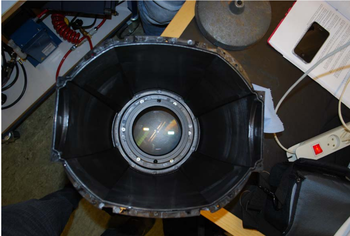
Photo 19. IPX5 No water observed inside the G-Spot Moving Head Profile.
