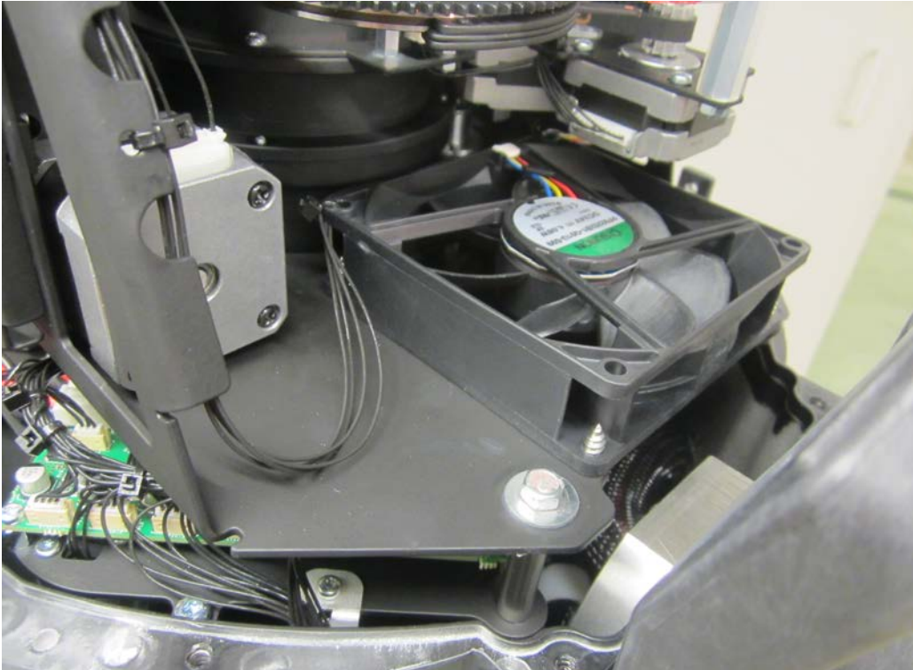
Photo 6. IP6X No dust observed inside the G-Spot Moving Head Profile.
