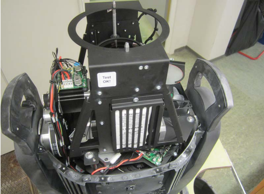
Photo 5. IP6X No dust observed inside the G-Spot Moving Head Profile.
