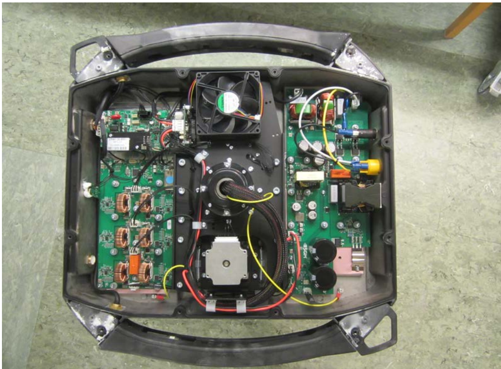
Photo 10. IP6X No dust observed inside the G-Spot Moving Head Profile.
