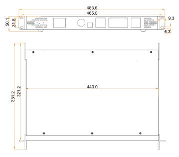
Tolerance: ±0.3 Unit: mm
