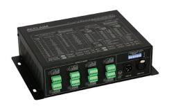
The **AL Driver 8 RGBW** is a high performance driver & power supply for 12V & 24V led fixtures. It offers 8 ouput ports to connect directly to fixtures such as the Flex RGB, as well as onboard DMX addressing
