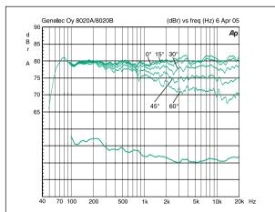
Figure 5: The upper curve group shows the horizontal directivity characteristics of the 8020B measured at 1 m. The lower curve shows the systems power response.
