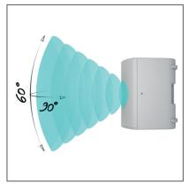
► The ellipsoid waveguide generates a directivity pattern of 90° x 60° to maximize X12 versatility in horizontal or vertical deployments.
