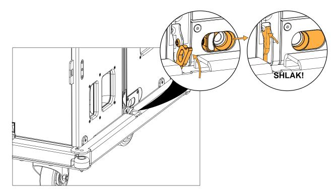
**4.** Disconnect a stack from the array on both sides.
