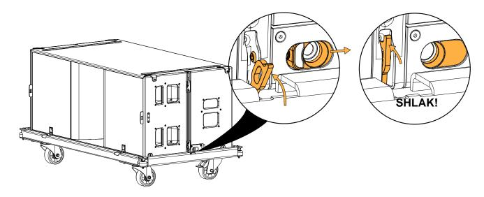
**3.** Place another KS28 on the assembly. Align the runners with the tracks.
