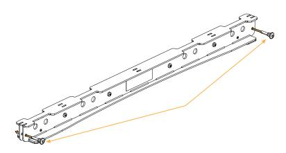
KS28-BUMP provides two sets of pickup points to choose from depending on the position of the lifting points. In addition, two sets of holes are available to implement a secondary safety.
