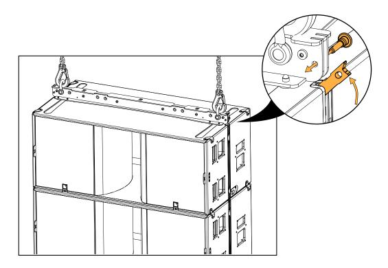
5. If KS28 is stacked on KS28-CHARIOT, remove the rigging arms from the chariot before lifting.
