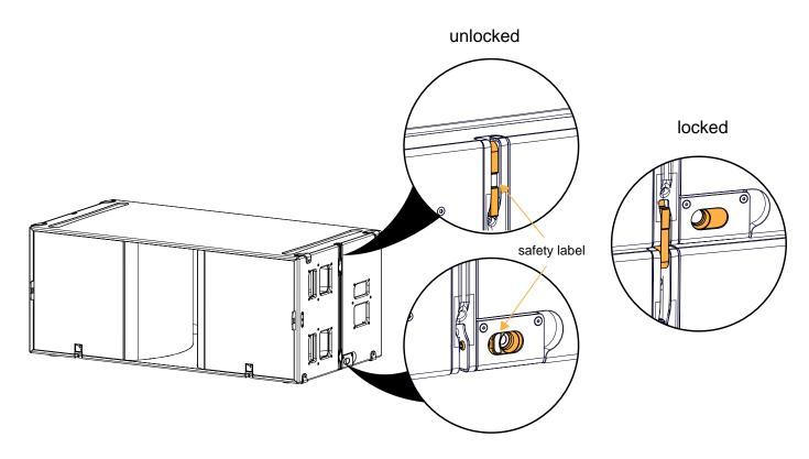
The rigging system allows securing enclosure arrays in stacked or on-end configuration.
