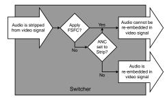
Figure 7: Audio Flow Through the Switcher
