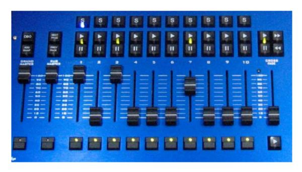
The playback area also contains a Grand Master, a Sub Master, Page Select buttons and a Manual Playback for taking control of Cue Stacks.
