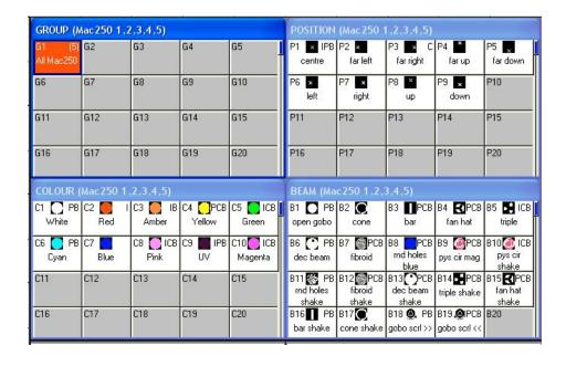
The highlighted window enables controls the soft buttons and rotary encoders. In each of the Windows the X and Y encoders control the most important attributes – Pan and Tilt in Position Window, Col Wheel 1 and Col Wheel 2 in the Colour Window and Gobo Wheel 1 and Gobo Wheel 2 in the Beam Window. In the Beam Window there are more than eight attributes to be controlled – these are accessed using multiple pages of encoders – by pressing the NEXT PAGE soft button.
