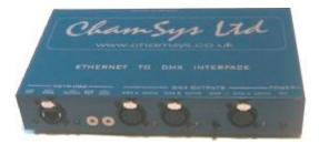
If you are using Ethernet to DMX512 conversion boxes then you will need to configure the boxes to respond to the correct ArtNet sub-net and ArtNet universe. With ChamSys 3 Universe Ethernet to DMX boxes you need to set up the two rotary switches to the correct values – the left one for ArtNet sub-net and the right one for ArtNet universe. The interface will then decode the three ArtNet universes starting from that ArtNet subnet and universe.
