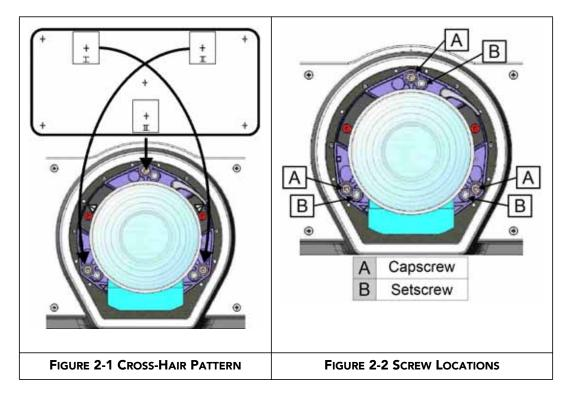
5. Fine tune the focus of cross-hair pattern I by adjusting the appropriate cap screw. Adjust until the cross-hair image is in focus with minimal flare.
