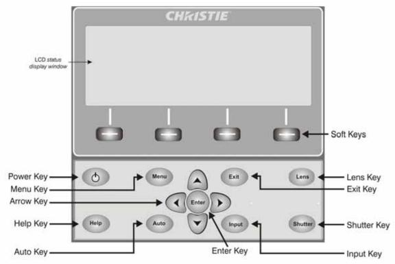
FIGURE 3-2 BUILT-IN KEYPAD
