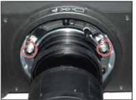
6. Use a 5mm hex driver to fasten the red security screws provided with the lens mount, or hand tighten the lens retaining screws attached to the lens.
