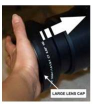
3. While holding the lens flat against the lens mount, rotate the lens clamp clockwise to lock the lens assembly in place.
