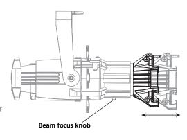
Step 3: Once the fixture is focused, tighten the beam focus knob.
