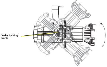
Step 1: Loosen the yoke locking knob. **Do not** remove the knob.
