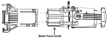
Step 1: Unscrew the beam focus knob from the loose lens tube.
