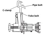
Step 2: Place the C-clamp on the mounting pipe, and then tighten the pipe bolt to secure it.
