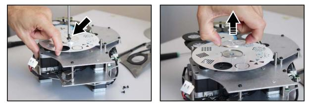
Figure 16: Releasing the static gobo wheel
