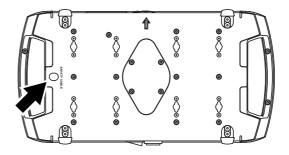
Figure 6: Safety cable attachment point
