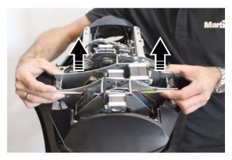
Figure 11: Removing the multi-module
