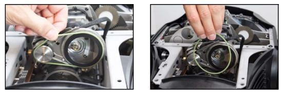
Figure 18: Removing the prism drivebelt
