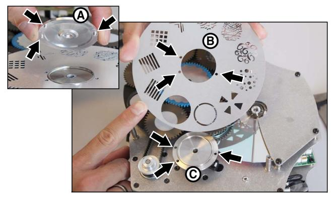
Figure 17: Static gobo wheel alignment
