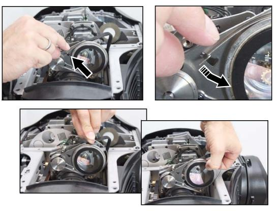
Figure 19: Removing the rotating prism
