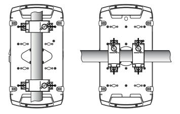
Figure 3: Clamp bracket positions
