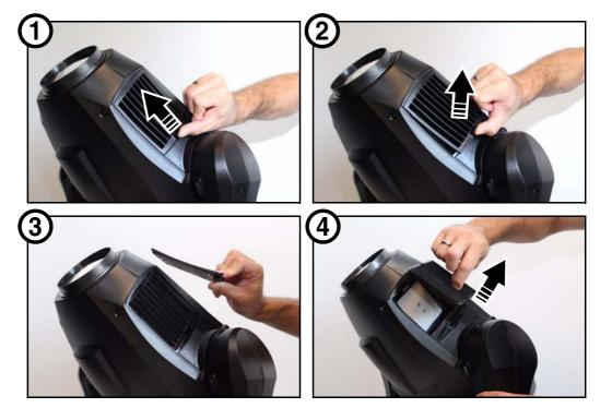
Figure 8: Releasing head air filter covers
