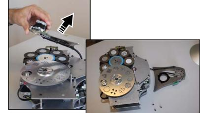
Figure 15: Moving the iris unit for access
