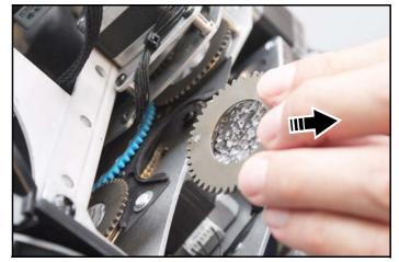
Figure 13: Removing a rotating gobo
