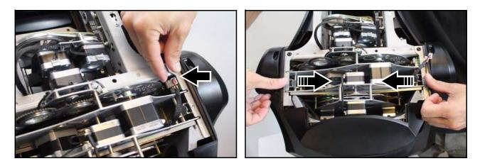
Figure 10: Releasing the multi-module
