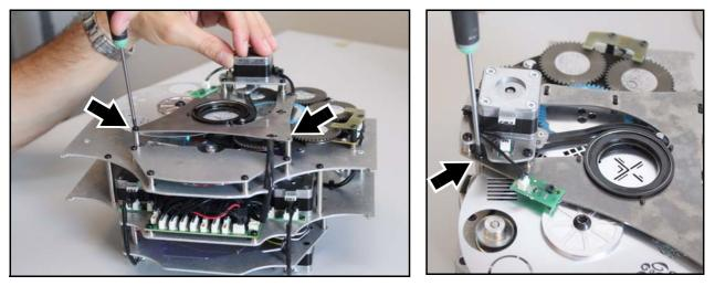
Figure 14: Releasing the iris unit
