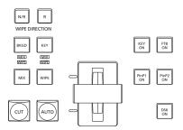
③ When the [FTB ON] button in the transition area is pressed, fade-out to the black screen is initiated for the length of the transition time that has been set.
