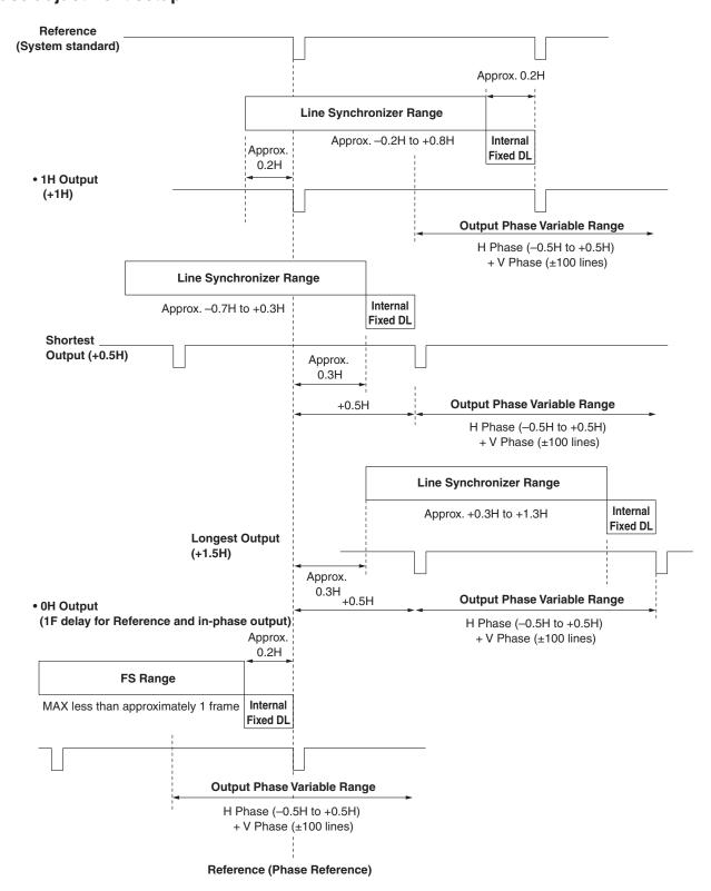
Line Synchronizer Range: Range for automatic phase adjustment.
