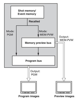
The resolution of the images output from the memories is lower than normal.
