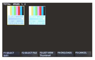
For Still thumbnails, the image is displayed in the upper portion, and the file name, KEY indicator, image size, and file date are displayed in the lower portion.
