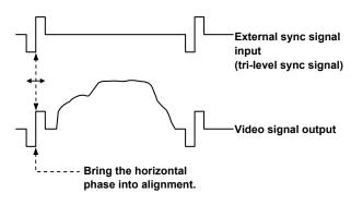
Example: When the tri-level sync phase is adjusted
