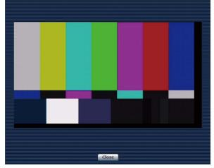
The IP video of the connected camera will be displayed. While the tally lamp is on, the area frame will turn red. When the tally lamp is off, the display area will return to normal. Operating the mouse wheel inside the display area allows you to use the plug-in viewer software's digital zoom. Windows
