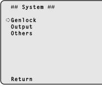
4. Press the <▲> or <▼> button to bring the cursor to [Genlock], and press the <>> button.
