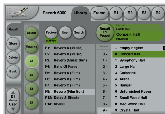
Fig 1. Location of Reverb 8 presets in your System 6000 MKII Engine Banks (F8 – Dec. 9)
